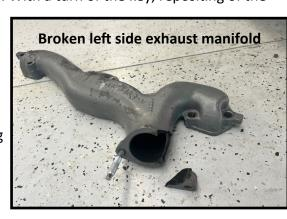
I searched the internet finding the replacement manifold. Doing the manifold replacement with the engine in place would prove challenging. With Mark's help we struggled to get the old manifold out and the new one in torquing all the manifold bolts to 48 foot-lbs. I connected the exhaust and replacement heat raiser this time carefully making sure not to over tighten the exhaust nuts.
